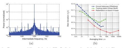
Fig. 2. Frequency stability of the 8.4 GHz RadioAstron downlink signal. (a) Phase-stopped signal spectrum (data recorded by the Effelsberg telescope, 2015/11/19). (b) Comparison of the frequency stability in terms of the Allan deviation of the signal recorded by a radio telescope (blue, circles) and a tracking station (green, diamonds). Allan deviation of the on-board H-maser obtained during laboratory tests (red, squares).
