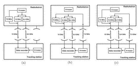
Fig. 1. On-board hardware synchronization modes. (a) "H-Maser". (b) "Coherent". (c) "Semi-Coherent". Note that, due to a fixed architecture of the RadioAstron on-board radio system, the 8.4 GHz tone and the carrier of the 15 GHz data link must use one and the same reference signal at any given time: either from the on-board H-maser or from the tracking station uplink.
